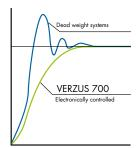
A wide force range, for Rockwell, Brinell and more. 1kgf up to 250kgf over load cell, closed loop system.
